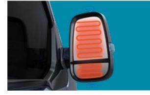
ELECTRIC HEATED SIDE MIRROR Heated electrically operated door mirrors ensure great rear visibility in all weather conditions.
